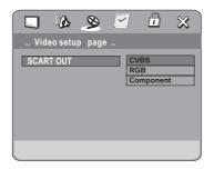
**CVBS**: Composite video output through the Scart output.
